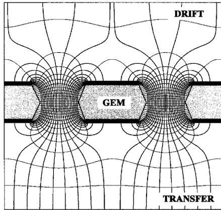
Fig. 5: Structure and fields in the gas electron multiplier
