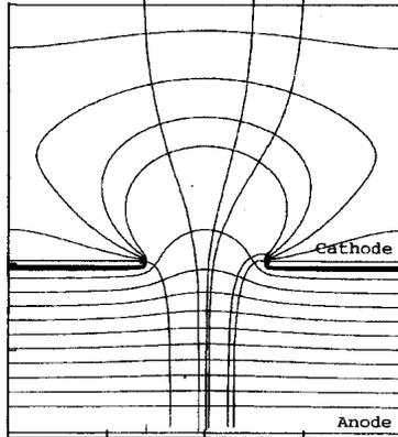
Fig. 4: Electric field in the CAT detector
