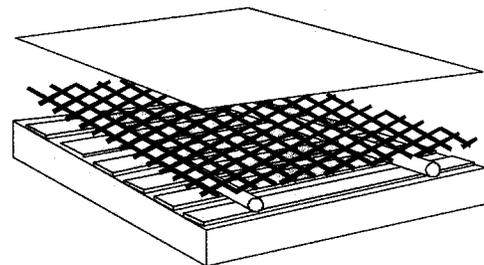
Fig. 3: Schematics of the micromegas
