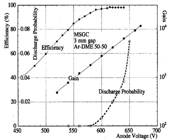
Fig. 2: Gain, efficiency for MIPs and discharge rate on alphas for the MSGC
