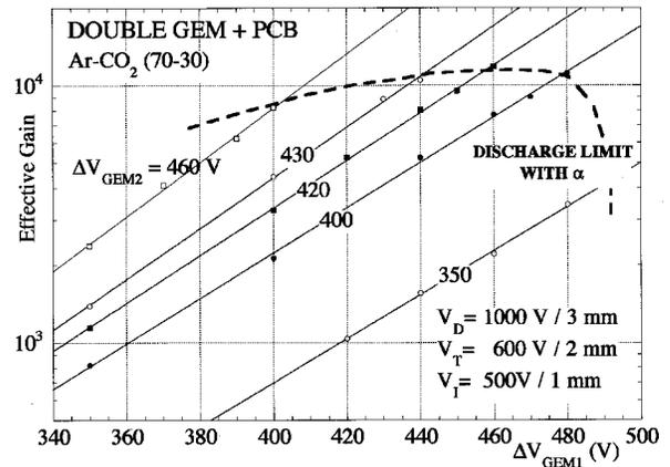
Fig. 6: Alpha discharge limit in the double GEM
