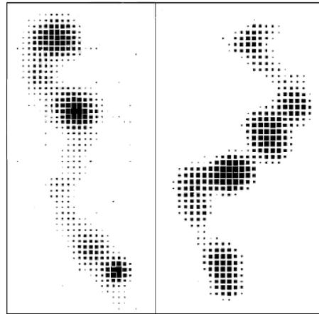
Fig. 12. Photoelectron tracks produced by 20 keV X-rays. Pixels are 100  $\mu\text{m}$  on the side.
