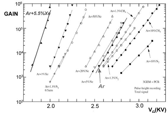
Fig. 10. Gain of a triple-GEM detector in noble gases mixtures.
