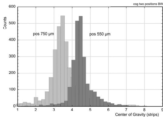
Fig. 11. Position accuracy of a CsI-GEM detector for single photons. Collimated UV source.
