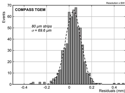
Fig. 5. Position accuracy for minimum ionizing particles.
