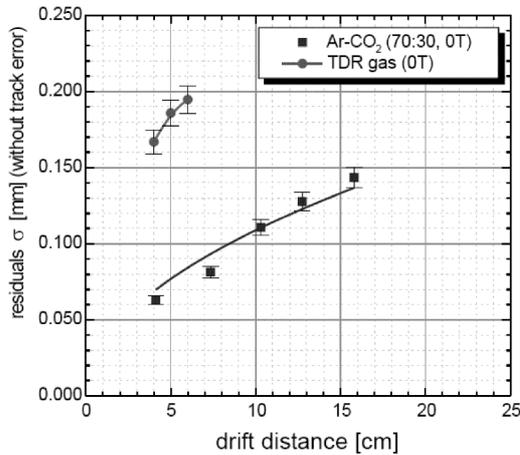
Fig. 8. Position accuracy for a single pad row in the GEM-TPC.
