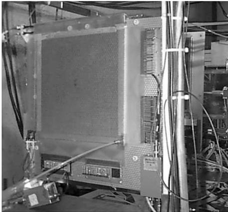
Fig. 4. A triple-GEM detector in the COMPASS experiment.
