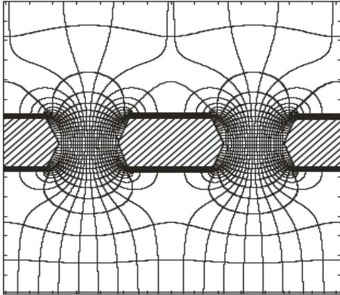
Fig. 1. Schematics and fields in the Gas Electron Multiplier.
