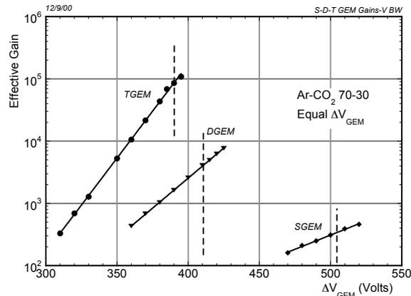
Fig. 2. Gain (full curves) and discharge limits on exposure to alpha particles (dashed lines) of multiple GEM detectors.
