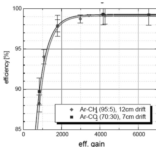
Fig. 7. Single pad row tracking efficiency as a function of gain in a prototype GEM-TPC, for two gas choices.
