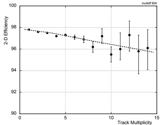
Fig. 6. Two-dimensional reconstruction efficiency as a function of track multiplicity.
