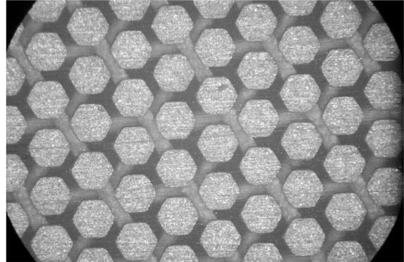
Fig. 9. The hexaboard readout; pads are about 400  $\mu\text{m}$  wide.
