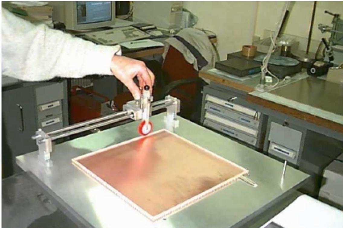
Fig. 18: View of the assembly table and epoxy-coating tool.
