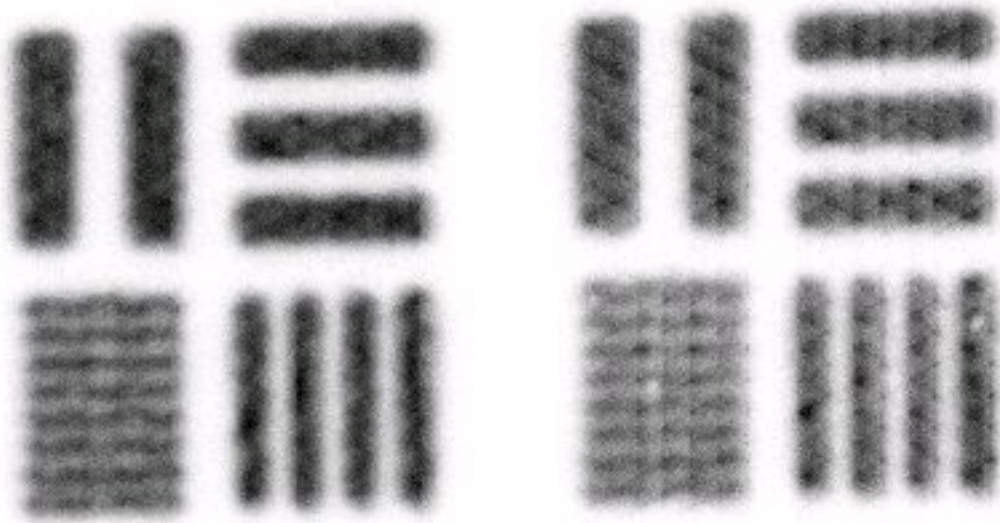
Fig. 7: Two-dimensional X-ray absorption pattern with a mask, 1 mm on the side, recorded with the hexaboard chamber. Left: the original pattern. Right: the one obtained adding up pairs of events to simulate high rates.
