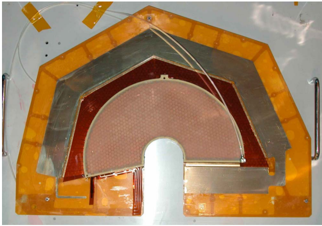
Fig. 9. The first prototype of the GEM assembled for a beam test.
