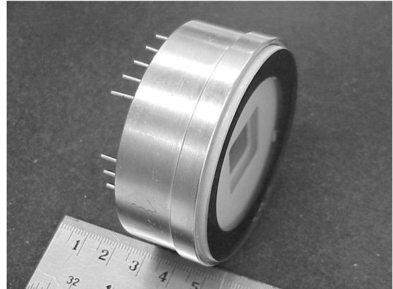
Fig.2 A photograph of the sealed GPM.
