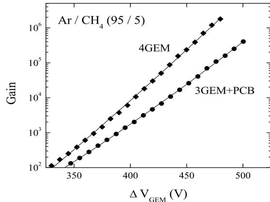
Fig.3 GPM gain as a function of the voltage drop across a single GEM, in 3GEM+PCB and 4GEM modes.
