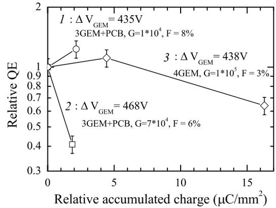
Fig.7 Induced ageing under irradiation in 3 ageing runs. Shown is the relative QE, normalized to the QE value at the beginning of each run, as a function of the accumulated anode charge in that particular run.
