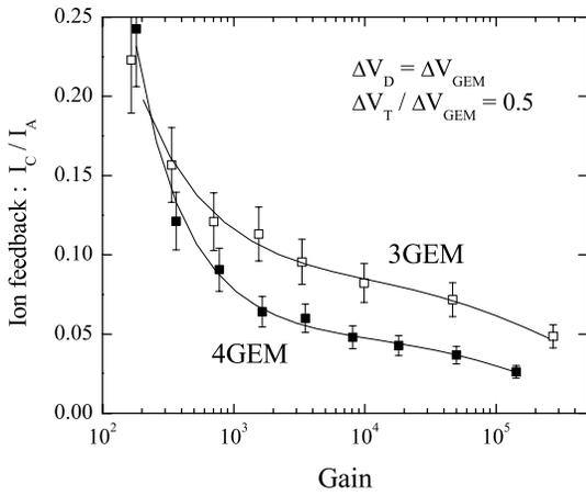
Fig.5 Ion feedback fraction to the photocathode as a function of the gain, in 3GEM and 4GEM modes.
