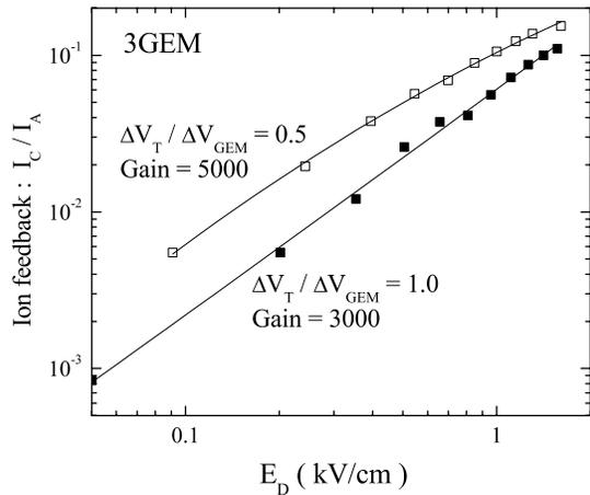
Fig.4 Ion feedback fraction to the photocathode as a function of the drift field, in 3GEM mode.
