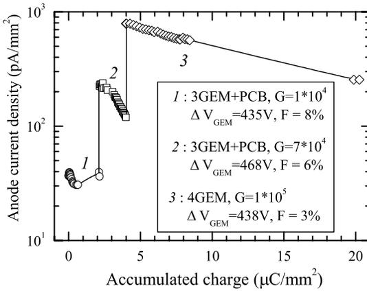
Fig.6 Induced ageing under irradiation. Shown is the evolution of the anode current density with the accumulated anode charge, in 3 ageing runs with different gains (G), voltage drops across a single GEM ( $\Delta V_{GEM}$ ) and operation modes. The ion feedback fraction to the photocathode (F) is indicated as well.
