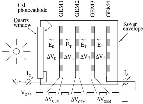
Fig.1 A schematic view of the sealed GEM photomultiplier (GPM).
