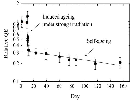
Fig.8 Long-term stability of the GPM. Shown is the evolution of the relative QE with time.
