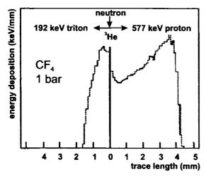
Fig. 4 The energy deposition along the proton and triton track in 1 bar  $CF_4$ .
