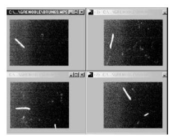
Fig. 7 Images of proton and triton tracks obtained with He(1bar)-CF<sub>4</sub> (400 mbar):  $V_{GEM1}=V_{GEM2}=V_{GEM3}=400V$ ,  $E_D=1kV/cm$ ,  $E_T=3$  kV/cm, CCD Binning 7×7, Texp.=10ms.
