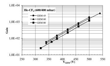
Fig. 1 GEM gains measured in He (600mbar)-CF<sub>4</sub> (400mbar) as a function of  $V_{GEM}$  for GEMs with 45, 60 and 80  $\mu$ m hole diameter.
