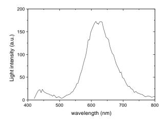
Fig. 3 Emission spectrum in He (600mbar) +CF<sub>4</sub> (400mbar) gas mixture measured at charge gain of 190 ( $\Delta\lambda$ =5 nm).
