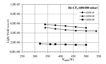
Fig. 2 Ratio of emitted light over secondary electron current versus  $V_{GEM}$  measured in He (600mbar) +CF<sub>4</sub> (400mbar) for GEMs with 45, 60 and 80  $\mu$ m hole diameter.
