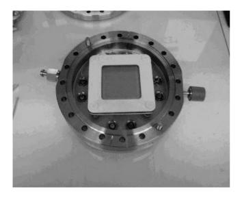
Fig. 6 Photograph of the detector with the entrance aluminium window removed, showing the stacked GEM assembly and transparent grid electrode.
